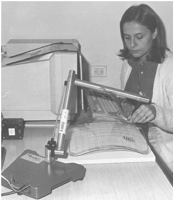
Fig.2 Digitizing a model by means of the SpaceArm
