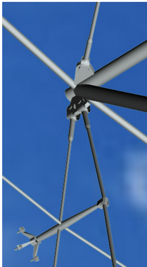
Figure 5a: Computer Image and Detail: Cable Net Connection to Roof Truss
