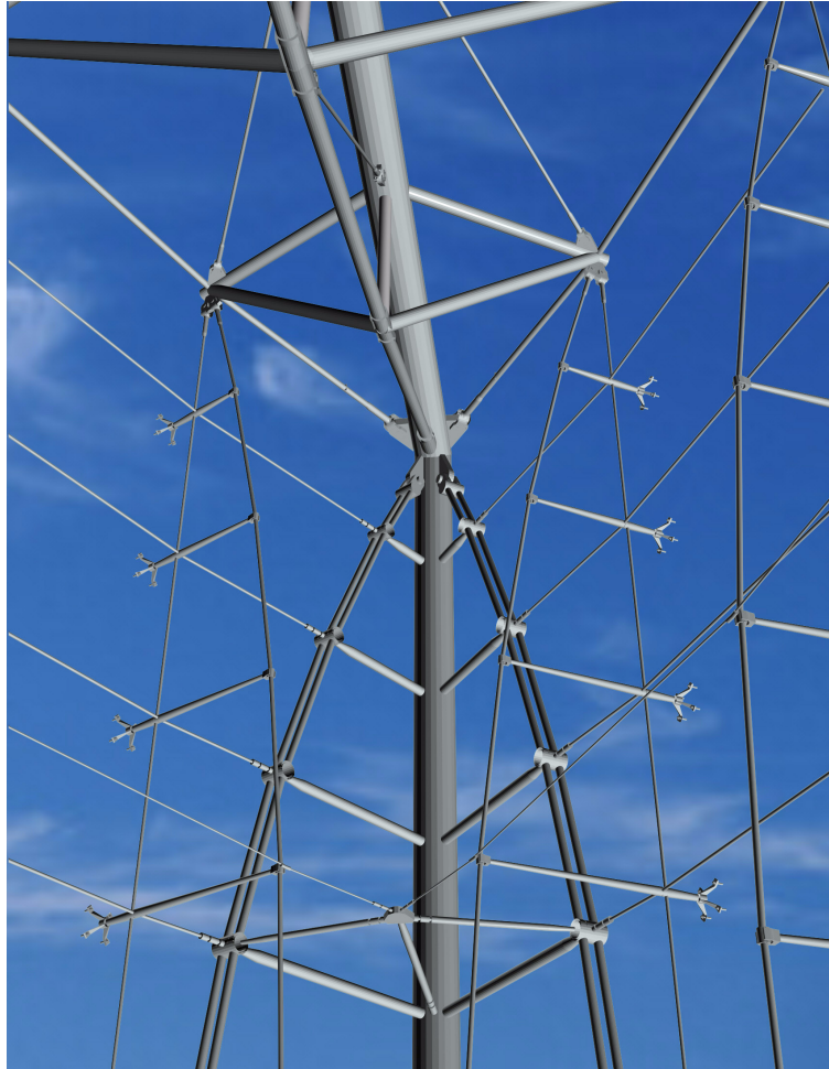
Figure 4: 3-Dimensional Computer Image of Upper Corner: End Post Truss, Roof Truss, Stabilizing Cables, and Cable Net Trusses
