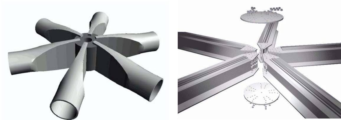
Figure 1: Connectors used in Reticulated Dome Structures.
