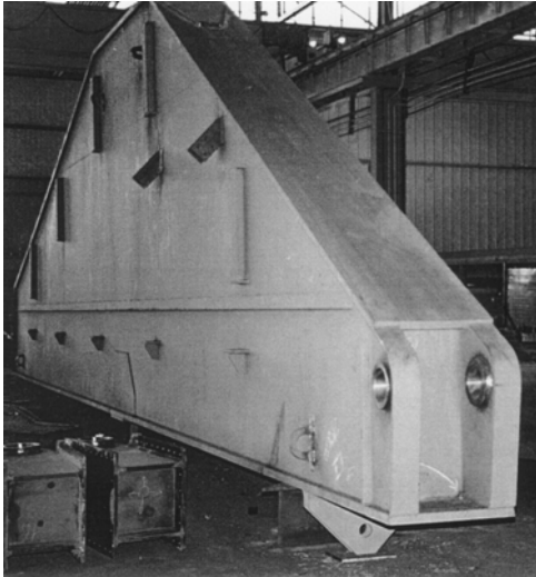
fig.07 sockets for pin connection sections
