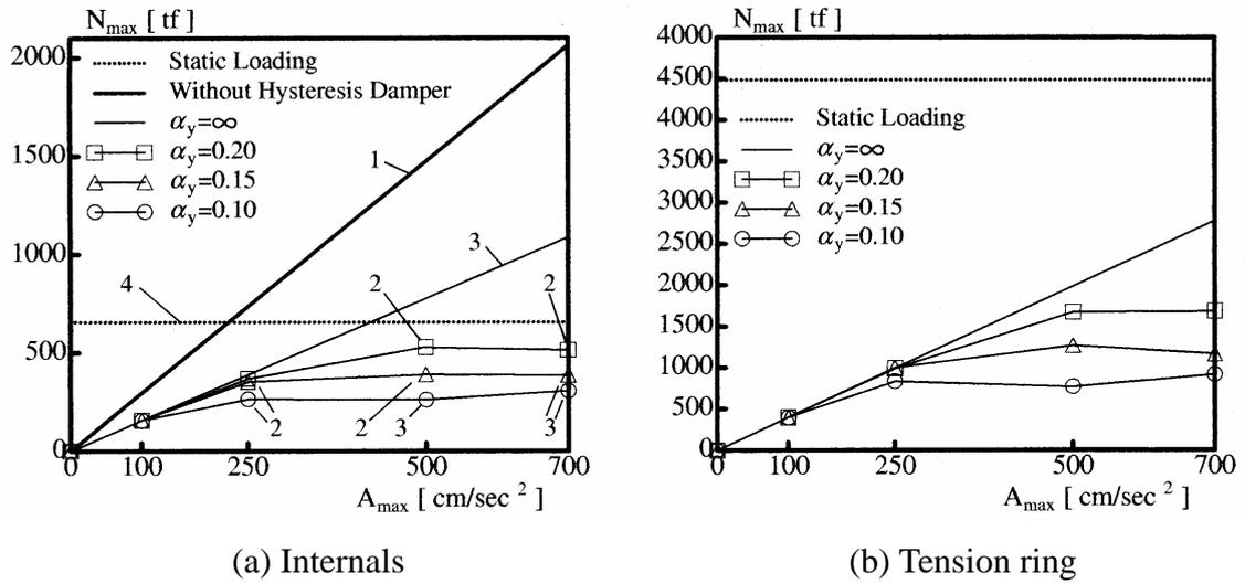
Fig.7 Relationship between the maximum axial forces of the dome and  $A_{max}$
