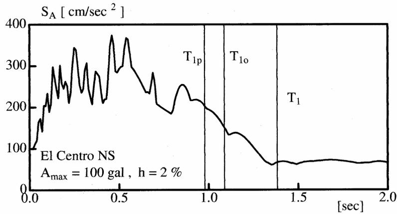
Fig.3 Acceleration Spectrum ( El-Centro NS,  $A_{max} = 100 \text{ cm/sec}^2$  )
