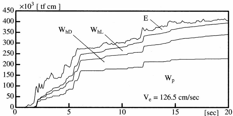
Fig.9.b Absorbed energy (  $A_{max} = 500$  cm/sec<sup>2</sup>,  $\alpha_y = 0.2$  )
