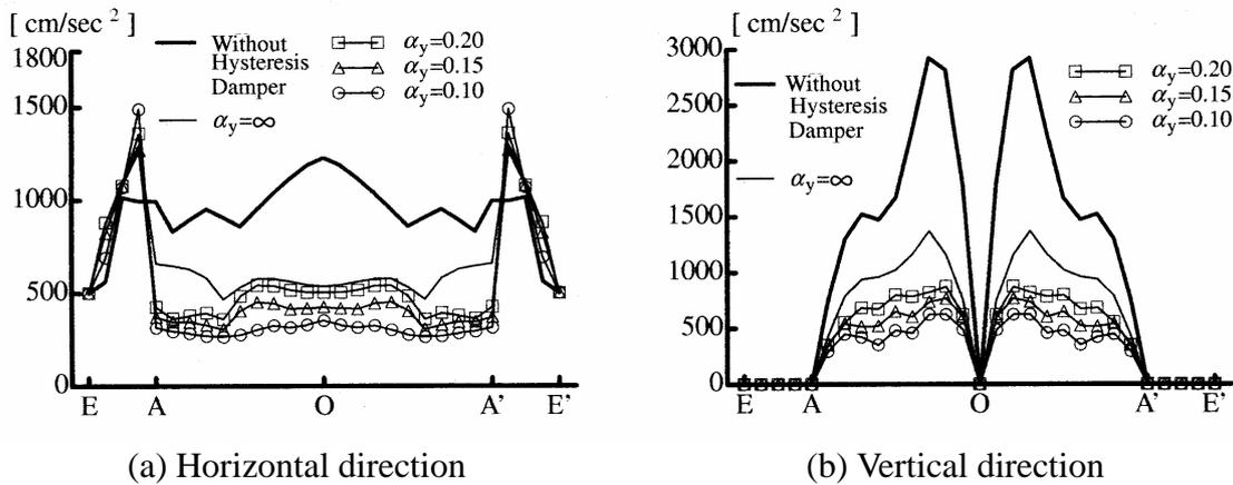
Fig.5 Distributions of the maximum response accelerations of the dome
