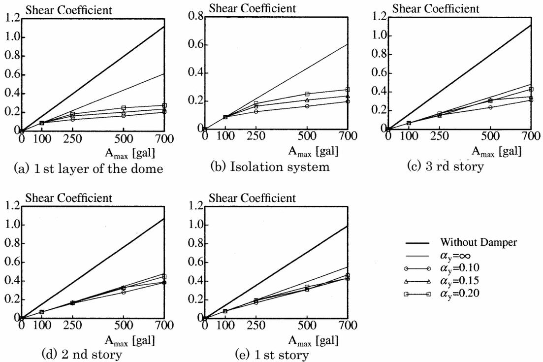
Fig.8 Relationship between response shear coefficients and input ground motion  $A_{max}$
