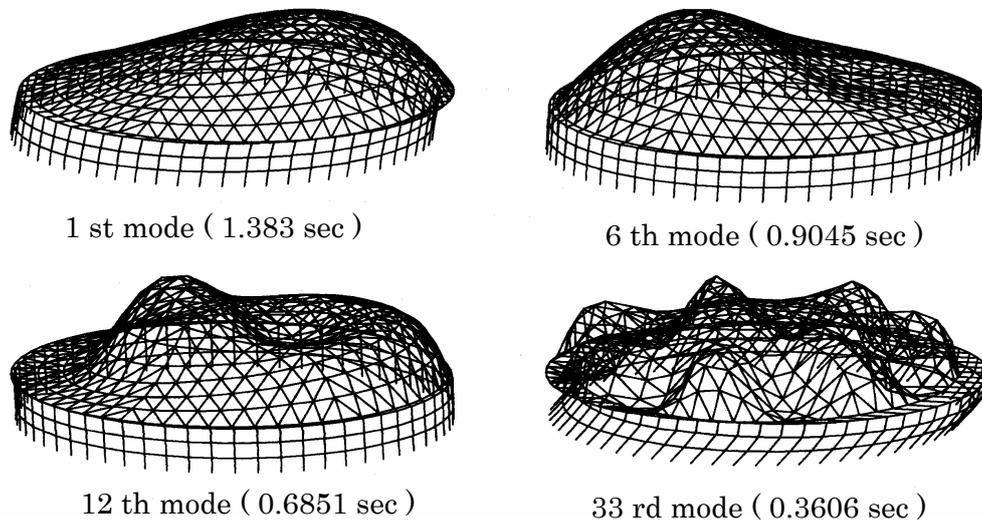
Fig.4 Vibration modes with hysteresis dampers
