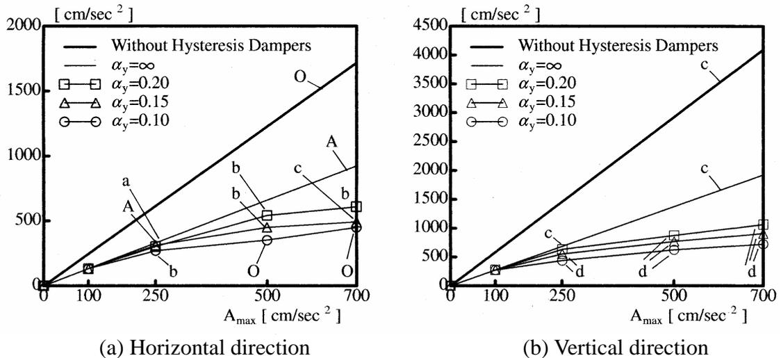
Fig.6 Relationship between the maximum accelerations of the dome and  $A_{max}$
