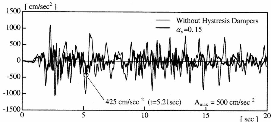
(a) Horizontal acceleration at the center of the dome
