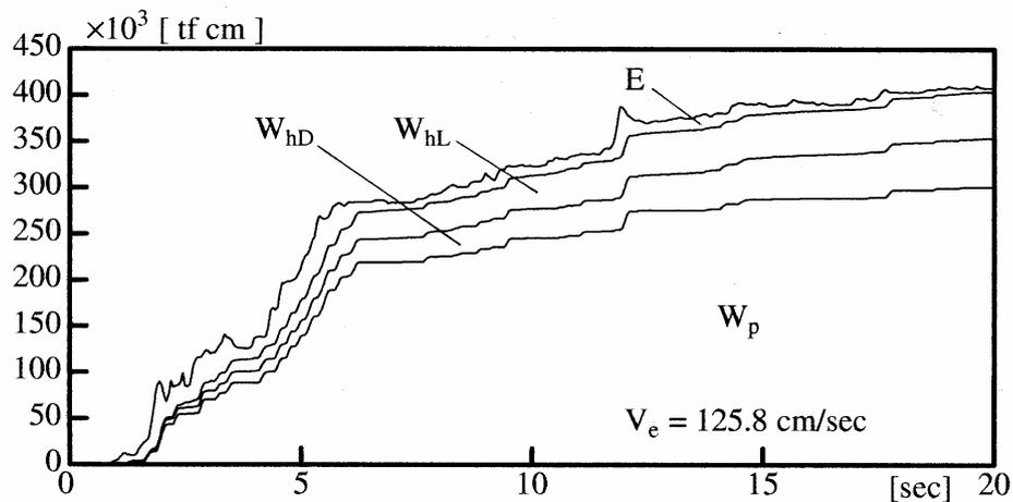
Fig.9.a Absorbed energy (  $A_{max} = 500$  cm/sec<sup>2</sup>,  $\alpha_y = 0.1$  )
