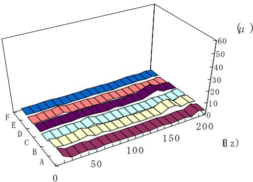
**Fig.7 Maximum absolute axial strains (Base isolated shell)**
