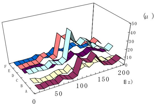
**Fig.8 Maximum absolute bending strains (Non-isolated shell)**
