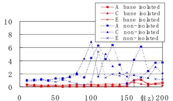
**Fig.10 Acceleration response magnifications at A,C and E (10-200Hz)**
