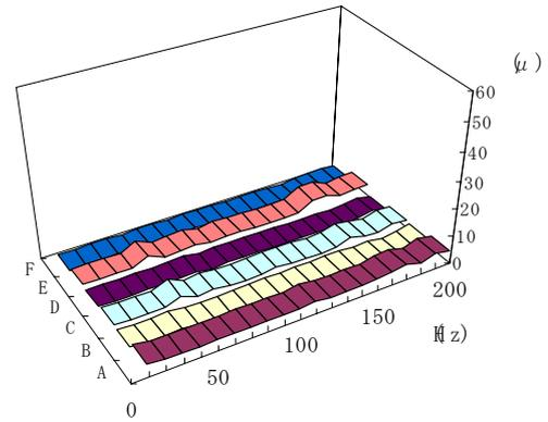
**Fig.9 Maximum absolute bending strains (Base isolated shell)**
