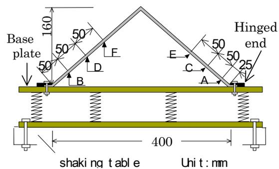
Fig. 2 Base isolated shell
