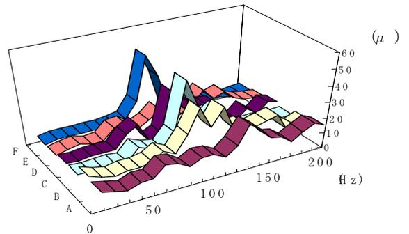
**Fig.4 Maximum absolute meridional strains on the Face (Non-isolated shell)**
