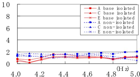
**Fig. 11 Acceleration response magnifications at A,C and E (4-5Hz)**
