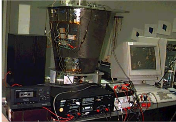
Figure 2: Sub-Scale Launch Vehicle Shroud with Active Acoustic Control
