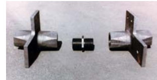
cast steel elements of central tension ring
