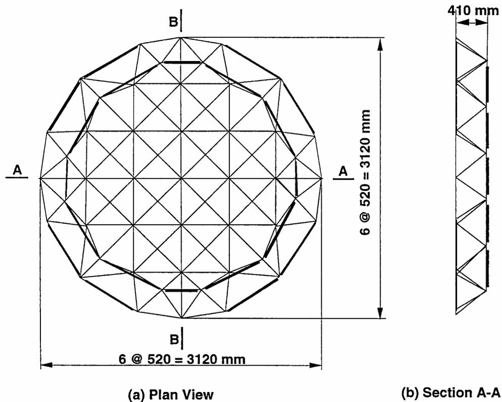
Figure 1 Planar layout (planar geometrical model) of SSBD 1
