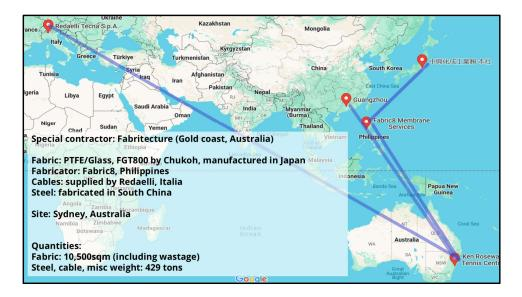
Site is in Sydney, Australia. Cables were manufactured in Italia, PTFE fabric manufactured in Japan, fabricated in the Philippines, steel manufactured in South China and then transported to site.
