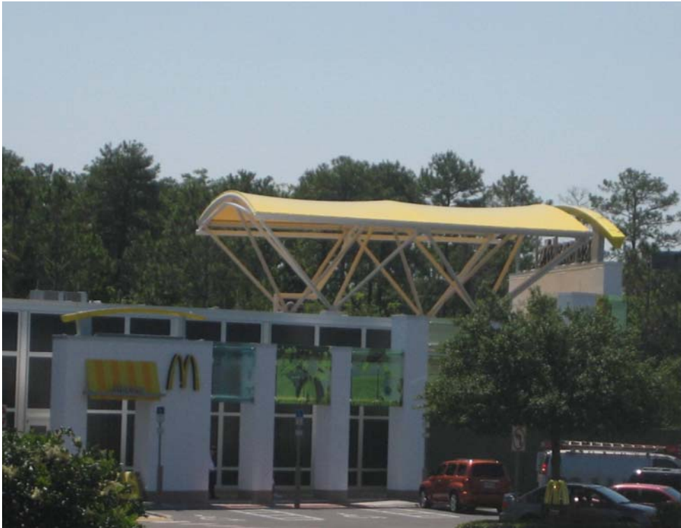
Figure 6. Coloured, backlit fabric for membrane structures. McDonalds, Florida.
