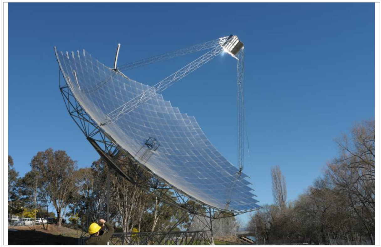
Fig. 11. First on sun tests with all mirrors uncovered
