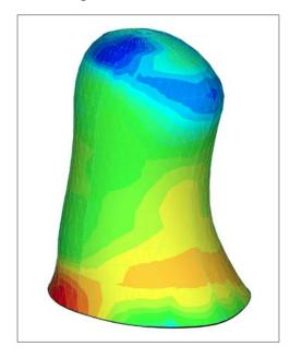
Tensys provided membrane engineering services to the foil fabricators Hightex GmbH. The challenge of the shape finding was to meet the architectural requirements whilst minimizing the foil stress and possibilities of wrinkling.
