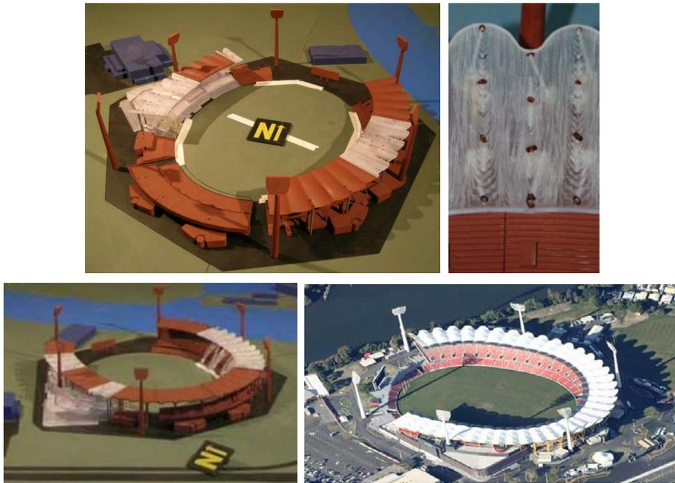
Figure 2: Photograph of Carrara Stadium wind-tunnel model and completed structure
