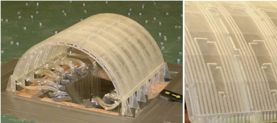
Figure 1: Rigid pressure model of a bulk storage structure
