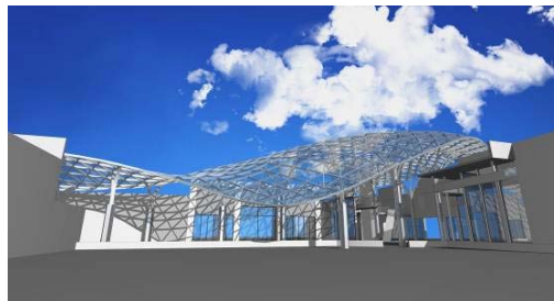
Fig. 3: Grasshopper generative model of Ballito Lifestyle Mall canopy imported into Archicad via Geometry Gym IFC translator
