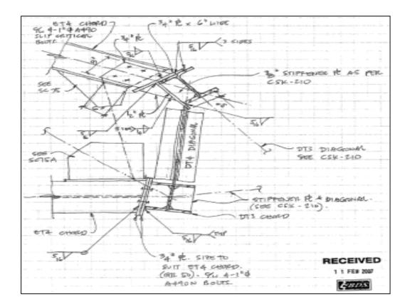
From the engineering's sketches BDS VirCon created a digital model and through a collaborative process it finalised the steel layout and developed the model in Tekla Structures<sup>2</sup> where all the elements were detailed in a parametrically perfect, data-rich model ("Detailing Model").
